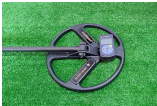
Fig. 1. Photo of the sensor and control unit of the X-Finder metal detector
