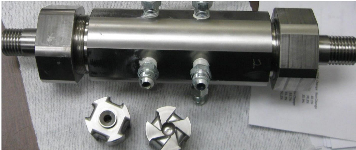
Fig. 5. The Fig. also shows a device for online mixing and homogenizing fuel mixtures before injection into the combustion chamber of a thermodynamic system, including internal components
