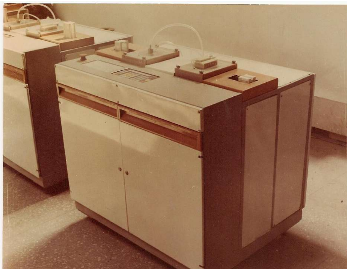
Fig. 8. The Fig. shows a flow-type automated production line for a full cycle of photolithography and chemical-mechanical processing on thin-film micro assemblies with a flexible organization of the local technological process within each unit included in the line; According to the TRIZ classification, the line is a technical system of a higher level of the hierarchy - a supersystem, each unit within the line is a technical system of a medium level of the hierarchy - a supersystem, and each working position is a technical system of a lower level of the hierarchy - a subsystem
