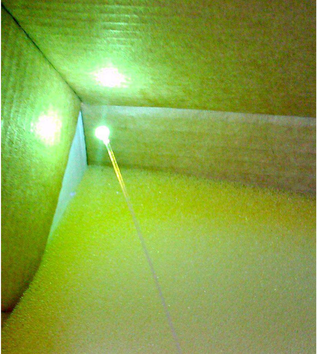
Fig. 9. The figure shows how the light from the phosphor falls into the corner of the box
