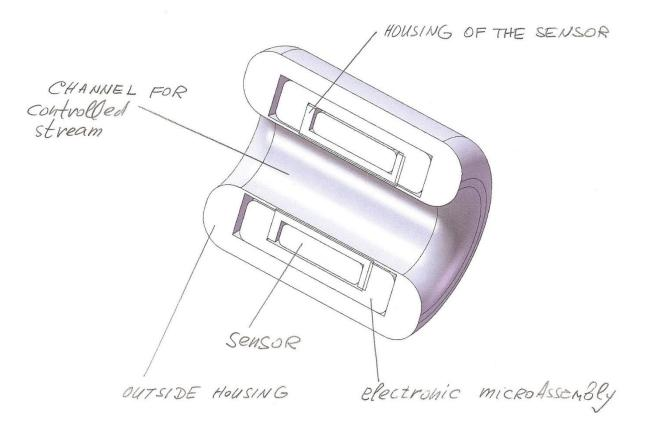
The sensor module has two main versions: the first version - for installation directly on the process pipeline before entering the working volume of the process tank, within the production premises; the second version-portable, designed to take samples of process solution or a mixture of process solutions from the dead zones of process tanks to the pipeline segment on which the sensormodule is installed. the module.
