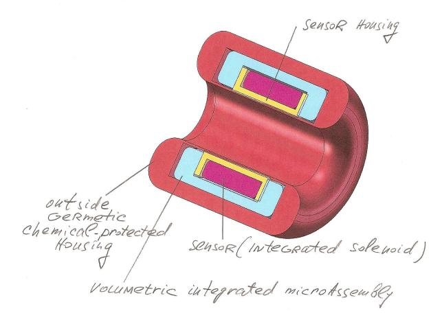
The height of micro-roughnesses at all internal surfaces of the sleeve is made minimal in order to, among other things, reduce the mechanical resistance to the movement of controlled liquids through the sleeve of the sensor module
