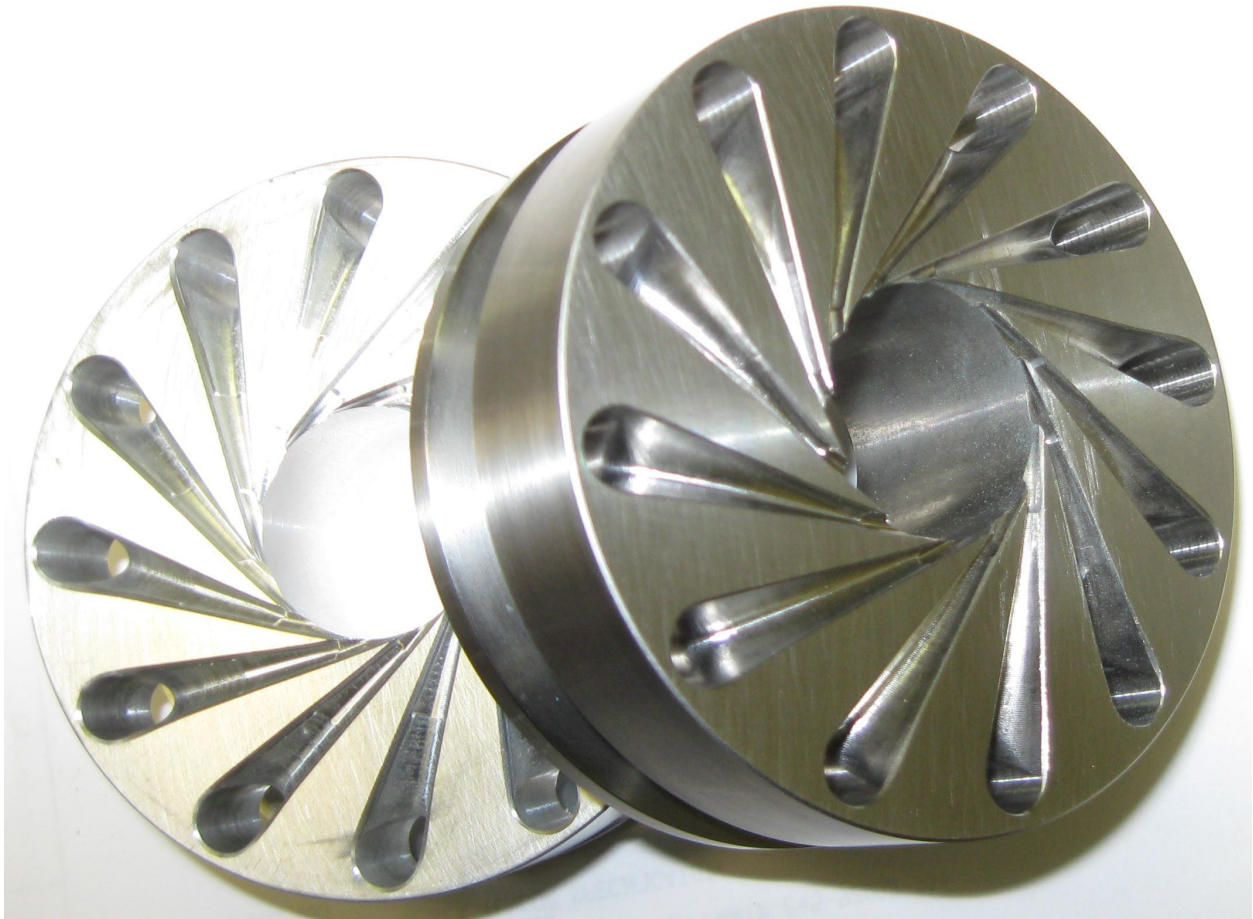
Fig. 1. The figure shows a vortex generator that forms a vortex tube in a flow of combustible gas
